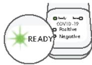
READY light should blink within 5 seconds. If not, press down harder on vial
